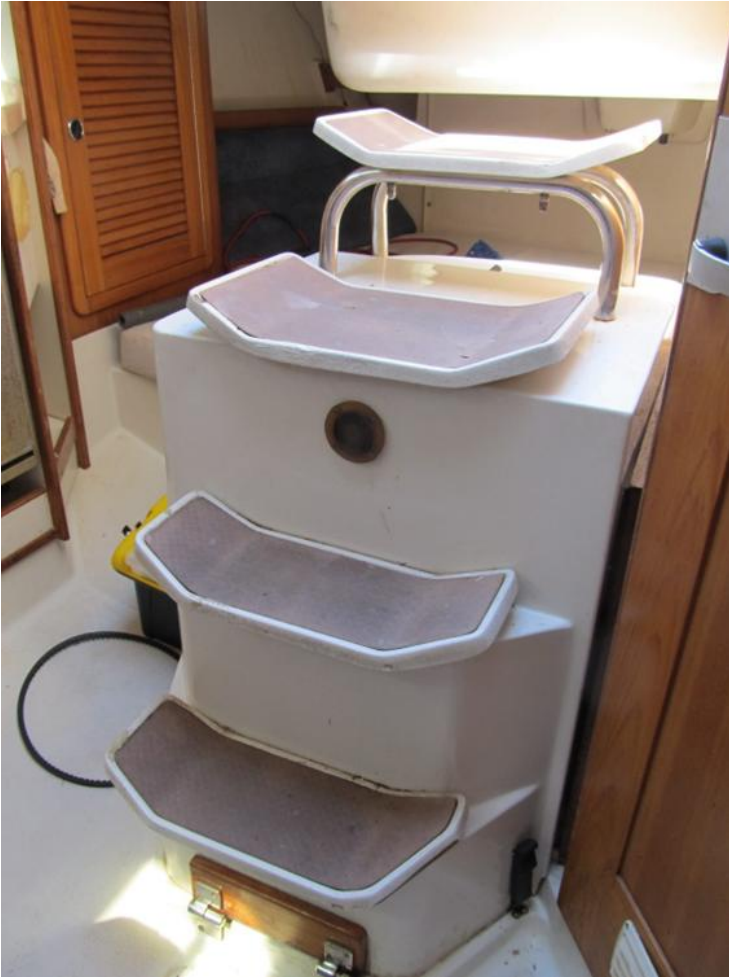
Entry steps with "Fire Port" in engine cover for Halation fire extinguisher.
