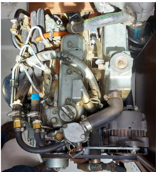
Engine with all the hoses on the pressure side replaced.
