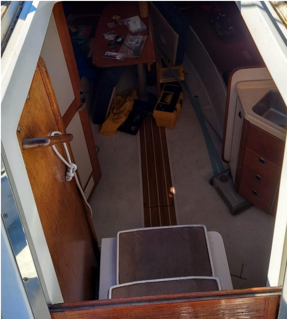
Cabin entrance with safety hand hold for steps.
